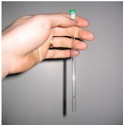
Figure 1. The NMR sample is prepared in a thin-walled glass tube - an NMR tube.
